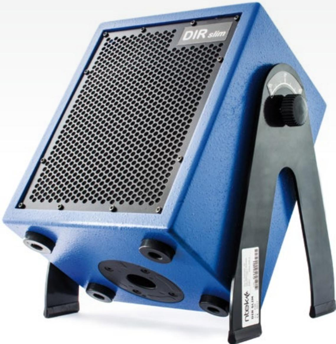
DIR SLIM - directional loudspeaker is a great instrument, solid and portable, able to produce a high noise level. For this reason and for his outstanding power and directivity is particularly suitable for sound insulation measurement and reverberation time. DIR Slim is perfect for AMG Mini systems as an alternative to OMNI dodecahedrons loudspeakers. DIR SLIM can be also used with other external amplifier sources, according with the system acoustic specifications.
