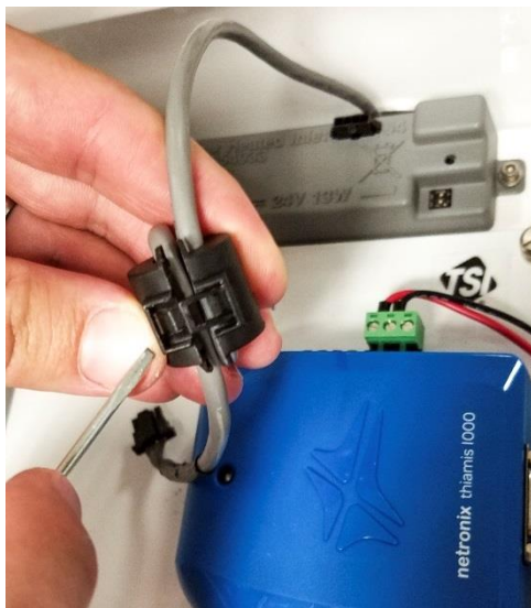
Figure 20: Removing ferrite clamp assembly
