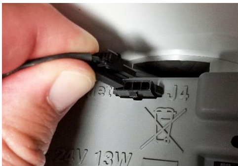
Figure 19: Disconnect heated inlet cable
