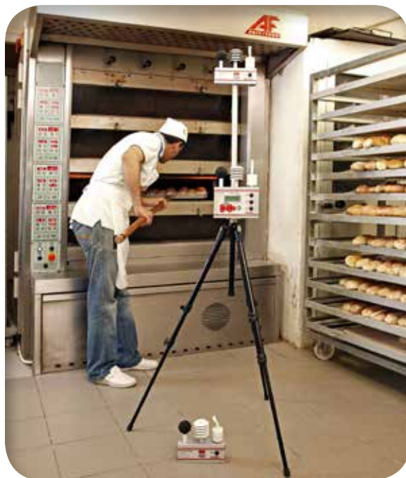
Three levels WBGT on the same vertical
