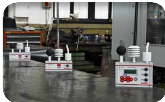
WBGT in three positions of the same environment
