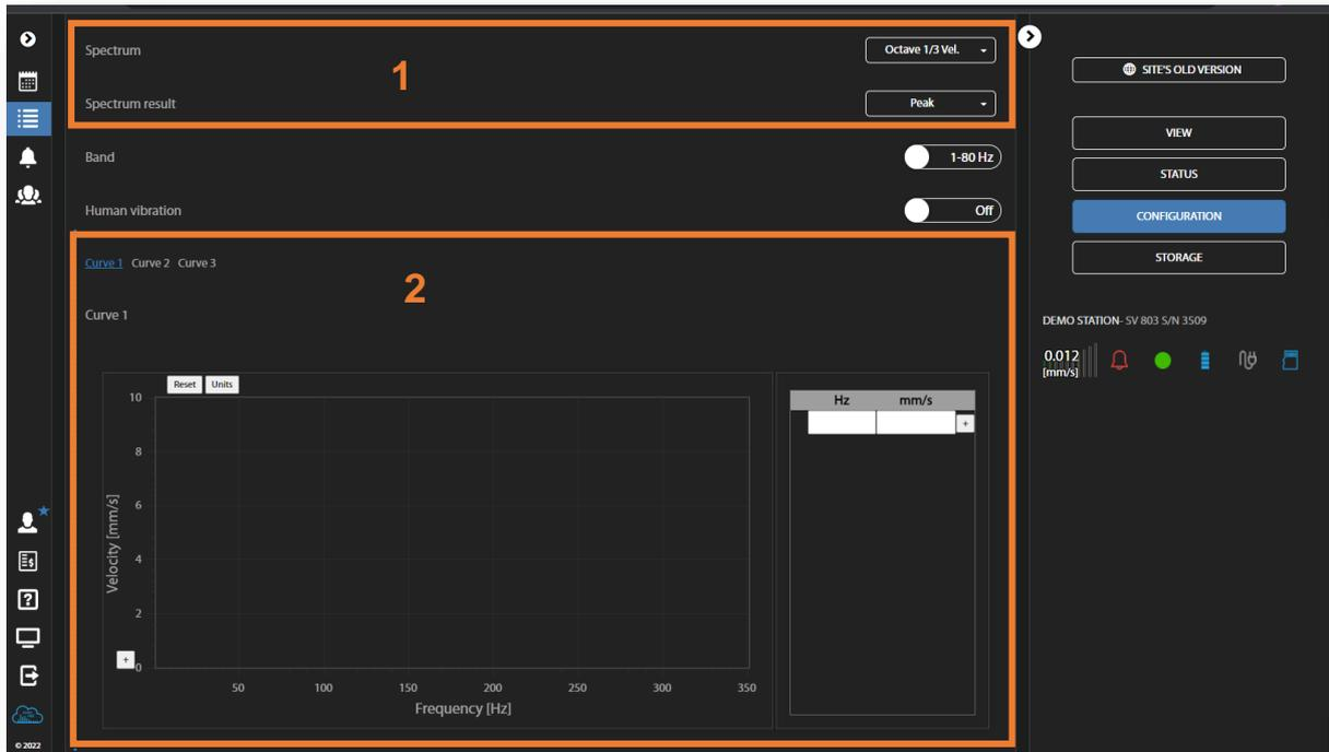
There are two ways to create a curve – using a table or a graph. Both ways complement each other. First, choose the curve you wish to create or modify (**Curve 1**, **Curve 2** or **Curve 3**).
