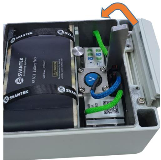
To disconnect the geophone cable, put the key on the connector and lean towards the battery.
