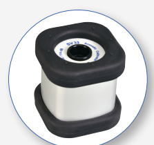
SV 35A Class 1 Acoustic Calibrator 94 dB / 114 dB at 1 kHz
