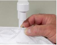
Step 5: Next, press down on the PortaPunch™ lever arm to engage the push nut onto the exposed point poking through the respirator and firmly push them together as far as possible.
