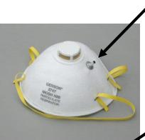
Correct probe location to left (or right) of valve
