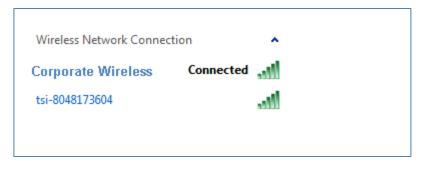
If the computer or tablet is connected to a wireless network, disconnect from it and connect to the PortaCount® Fit Tester. You will be prompted for a network security ID. By default this is the same as the wireless network connection name. Once these steps are complete, launch the FitPro™ Ultra Fit Test Software and the PortaCount® Fit Tester will be listed on the Connect screen with a Wi-Fi® connection type ...
