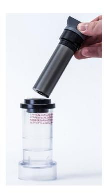
11. Insert the alcohol cartridge into the cartridge cavity of the PortaCount<sup>®</sup> Fit Tester. It should slide in with little effort; DO NOT force it. As you approach full insertion, firmly twist the alcohol cartridge clockwise until it locks into position.
