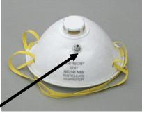
For Respirators with an Outer Mesh—install the probe normally as if the mesh was not present. The sampling probe and push nut will seal properly right through the mesh.
