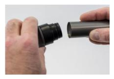
After separating the two halves, push the alcohol wick out of the wick retainer cap from the opposite end. **DO NOT** use a pencil point because bits of lead could break off.
